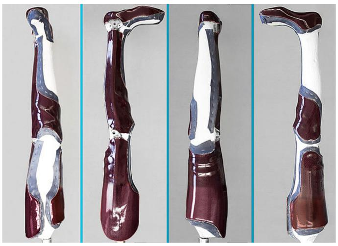
Remove all laminate parts which are no longer necessary. Then, you can remove the orthosis parts from the model.
