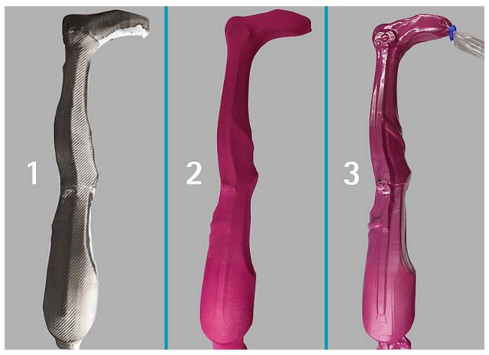
In order to secure the reinforcement layers, pull a decorative fabric (2) or a PA reinforcement stocking (for a carbon look) over the model (1). Thus, the PVA film tube can easily be pulled over as top film layer (3).
