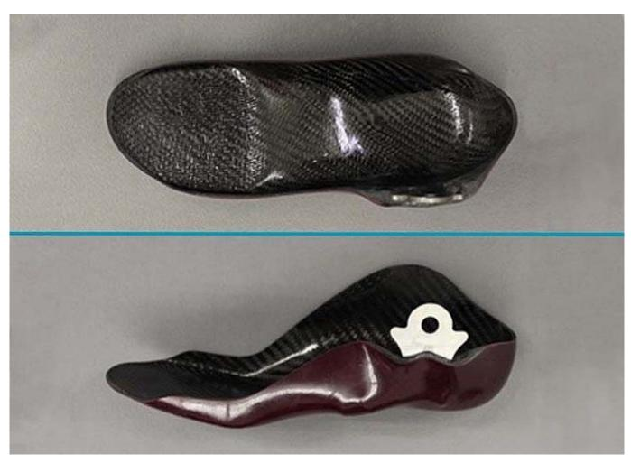
Grind the edges of the orthosis parts (e.g. with a belt grinder). However, it is essential to avoid predetermined breaking points in the metal!
