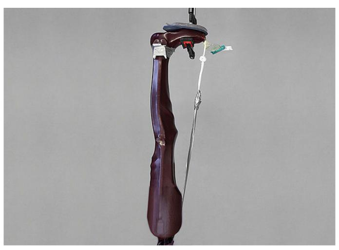
Let the model harden over night (at least 10 hours), under vacuum and at room temperature. Please note! Also follow the processing instructions for epoxy resin.
