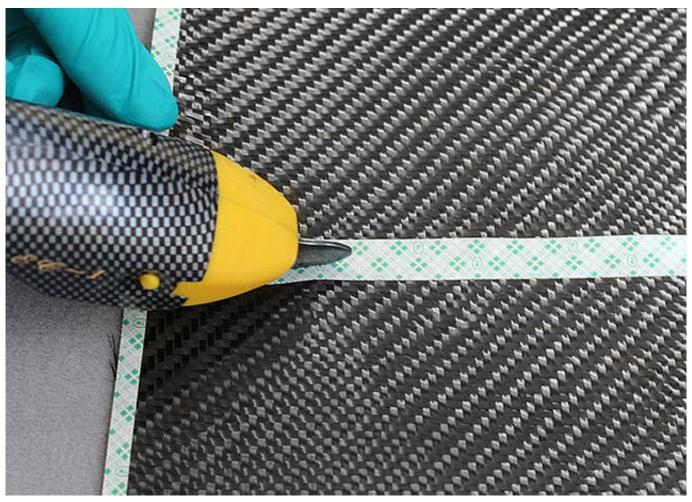
Please note! Due to the materials' characteristics, always wear nitrile gloves while working with carbon or aramid fibre fabric.
