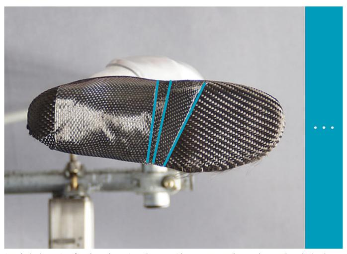
Attach the layers in a fan-shaped way, in order to avoid unnecessary edges and strengthen the heel area.
