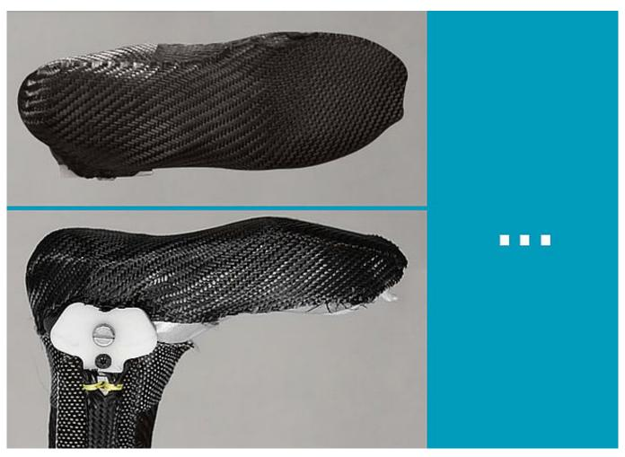
Continue reinforcing. Use as many layers carbon fibre fabric and band as you need for the foot piece (this is an exemplary picture).
