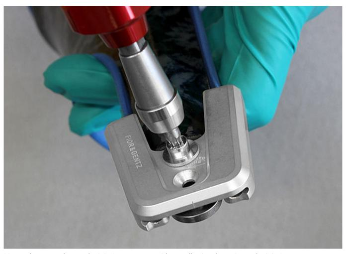
Mount the cover plate to the joint's upper part without adhering them. Press the joint's upper part to the cover plate as described in the instructions for use. Continue assembling the joint as usual.
