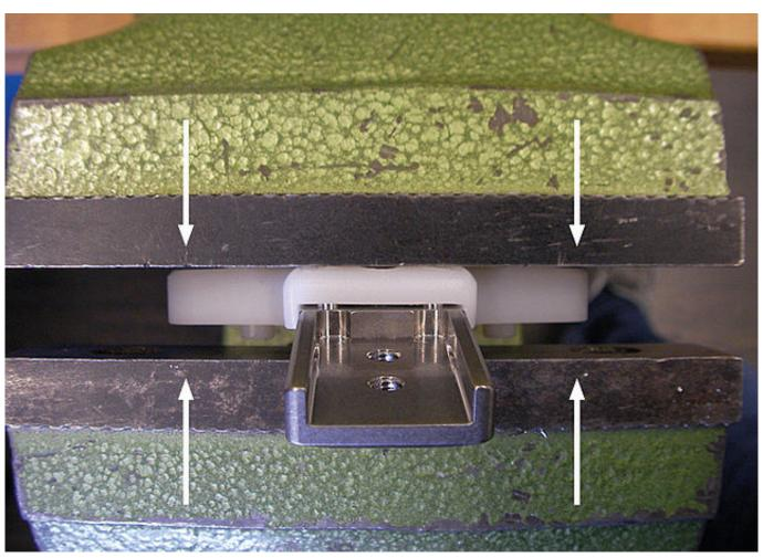
Press the assembly/lamination dummy to the joint's upper part in a vice with plain jaws until there is no opening left between them.
