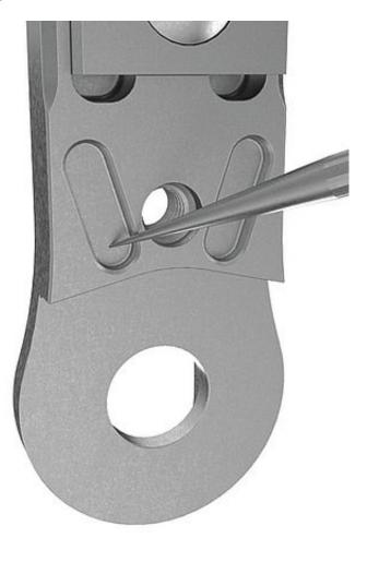
Clean the grooves of the joint's upper part thoroughly, otherwise the feather keys with pin cannot be mounted correctly. This is important, as incorrectly mounted feather keys with pin are very hard to remove.
