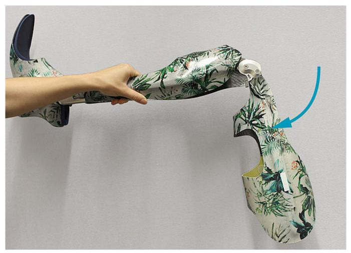
Check if the system joint moves freely. Bring the system joint in extension. In order to check the flexion, hold the orthosis in a horizontal position and then let go of the femoral shell. The femoral shell should smoothly fall downward up to the maximum possible flexion angle. If the system joint does not move freely, mount the next thinner sliding washers.
