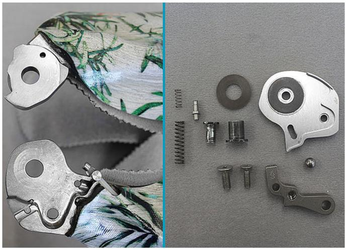
Disassemble the system joint completely.
