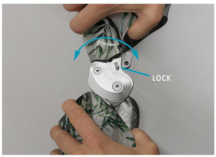
Check if the lock function works without play. If there is play, new locking parts are necessary.
