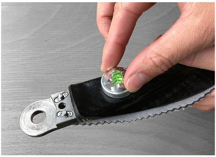
Clean the areas to be adhered. Mix a small amount of AGOMET® F330. Adhere the spirit level onto the prepared area. Mind the safety data sheet and let the adhesive cure sufficiently.
