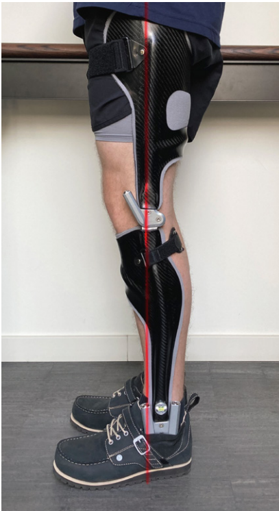
Fig. 5 Static alignment of the test orthosis on the test subject.
